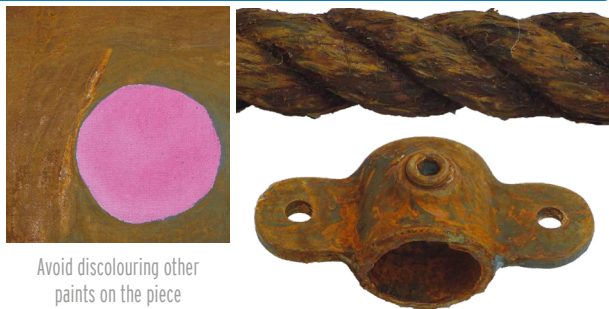
Objects rusted with the HATO@Rust system; above a piece of fibre rope, below a galvanised Key Clamp.
