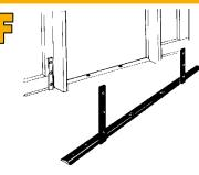
**Sill Iron** Used to provide strength to door flats. They are made-up to suit your requirements, from a flat steel bar with a rounded top section. They should be ordered by stating the distance between the lugs. On a 3 x 1" timber flat with a reveal around the door this
