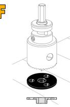
Round Boss Plate This product was suggested to us by Alan Cohen and we agreed that it would be very useful to speed up setting boss plates on stage. A 51 mm hole saw will neatly cut through the usual hardboard stage cladding. The hardboard can be discarded and the plate set in the hole. The finish is black powder coated. Size: 50 mm diameter x 3 mm thick [10 mm to base of boss]. Fixings needed: Three No.8 or No.10 [4, 4.5 or 5 mm] csk wood screws. Weight: 52 g.
