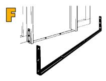
Reveal Iron Like the Sill Iron the reveal iron is used to provide strength to a doorway but this time the lugs are at right angles to the sill and are bolted through the door reveal. They are made to order and the measurement we require is the distance across the outside of the
