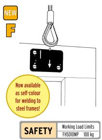
Opera House **Grummet** Flints makes these fittings for the Royal Opera House. They allow the ferrules on made-up wire ropes to pass through the 17 x 45 mm slot. They are quicker to use than the Two-part Grummet and considerably stronger than Open Grummets. Black powder coated finish. Fixings needed: 4 off 5 mm csk machine screws and T-Nuts. Now available as self-colour for welding to steel frames.
