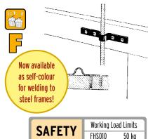
**Grummet** A conventional grummet for securing flying wires to the top of flats. This cheap strong fitting should always be fixed with two machine screws and two wood screws. The grummet can be subjected to significant loads during the initial raising of the flats. Once raised, virtually all the strain will be transferred to the bottom rail. The finish is black powder coated. Size:
