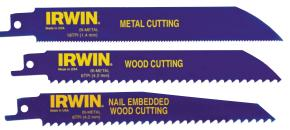
Reciprocating Sabre Saw Blades These bi-metal blades fit DeWalt, Bosch, Black and Decker, Hitachi, Metabo, Makita and Skil. The metal cutting blades will swiftly cut through metals 1.5 - 10 mm thick including non-ferrous, pipe conduit, steel sheet and stainless steel. The wood, and metal/wood [nail embedded] blades will rapidly cut wood 5 mm and thicker. See page 280 for the 18 V cordless DeWalt Reciprocating Saw.
