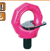
**Starpoint VRS F** Often referred to as "Pink Ladies". The pull on most eye bolts has to be restricted to the plane of the eye but the Starpoint VRS adjusts through 360° to align with the direction of pull. The star-shaped design and striking fluorescent pink powder coating clearly distinguishes it from other eye bolts. Each bolt has a clear WLL
