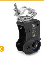
End of Line Unit This unit forms part of the circuitry which proves electrical continuity in the cabling. Only used in conjunction with the Sensing/DMX Firing Unit. The unit has three switches, all of which should be on for a single chain of Kabukis. Individual switches should be used when two or three chains of Kabukis are used in conjunction with the splitter box. A green LED on the unit indicates the cables are correctly connected.
