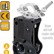
EK2 Electro Kabuki **Units** This award-winning design will reliably release weights of up to 50 kg. It can be used to drop items such as backdrops, dummies or cables on cue from a remote position. The load can be released as a vertical drop or at angles up to horizontal. The item is attached to a hook arm which pivots free when the magnet is energised.
